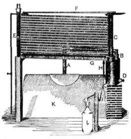
upright tubes at either side are made of stoneware, the connecting tubes are of thin glass. The pipe A, made of stoneware, carries the nitric acid vapors from the retort into the pot B provided with a stopper, D, which is taken out if frothing should occur and allows the froth to escape without danger of filling the condenser. The vapors pass up into C and are distributed
